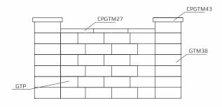
Drawing no.4 - Laying the wall "block over the block"
