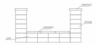
Drawing no.3 - Laying the wall alternately
